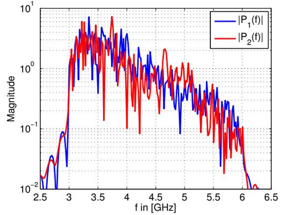
Fig. 4. Normalized spectrum of optimized precoding pulses  $p_1(t)$  and  $p_2(t)$  for region 9 and 17, respectively.
