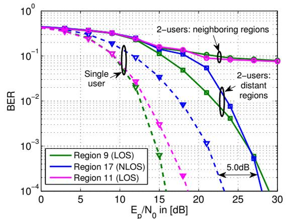
Fig. 6. Average bit error rate for precoding regional channel knowledge.
