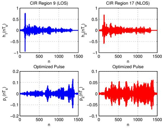
Fig. 2. Channel impulse response vectors from region 9 (LOS) and 17 (NLOS) and resulting precoding vectors for two nodes.
