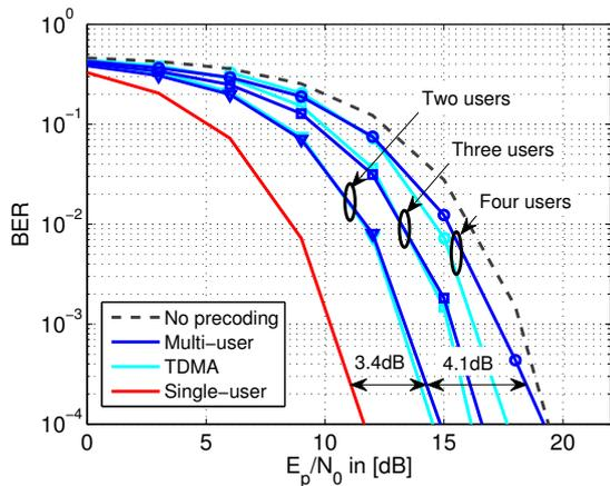
Fig. 5. Average bit error rate for precoding with full channel knowledge (Region 9, 17, 20, and 11).
