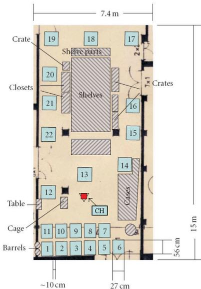
Fig. 3. Floor plan of measurement area
