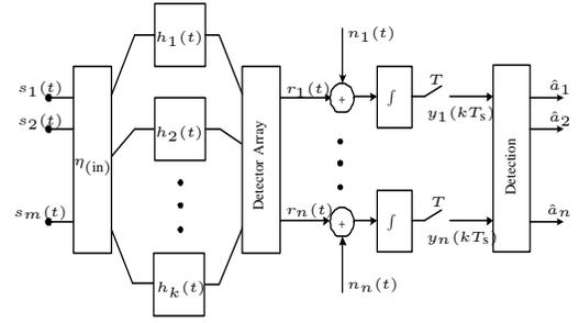
Fig. 2. Optical MIMO channel model and simple receiver, the noise is due to thermal noise in the electronics.
