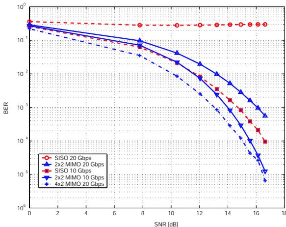
Fig. 4. Bit error rates vs. electrical signal-to-noise ratio for different transmission schemes. error curves by Monte Carlo simulations for different settings.
