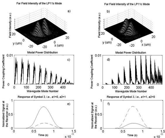
Fig. 3. Far field and modal power distribution: (a) Far field intensity of the  $LP_{11}^s$ . (b) Far field intensity of the  $LP_{11}^c$ . (c) Modal power distribution of the x-polarized modes. (d) Modal power distribution of the y-polarized modes. Signal at the different detectors after 1m waveguide caused by the input symbol: (e)  $a_1 = 0, a_2 = 1$  (f)  $a_1 = 1, a_2 = 0$
