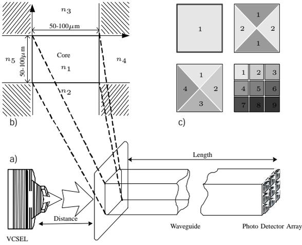
Fig. 1. (a) System Overview with VCSEL, waveguide and photodetector array. (b) Schematic of the five separable dielectric regions of a rectangular dielectric waveguide model. (c) Geometry of possible detector arrays.
