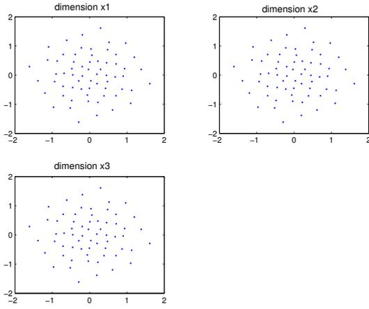
Fig. 2. Outer code: chirp matrix; all 64 coded vectors for block length  $N_C = N_I = 3$  and 4QAM
