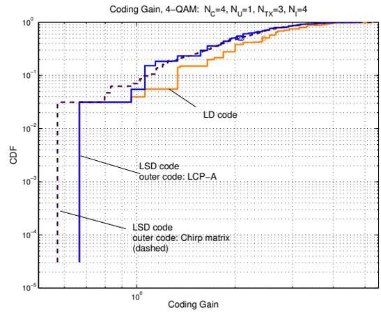
Fig. 9. CDF of coding gain: Comparison of LD and LSD codes
