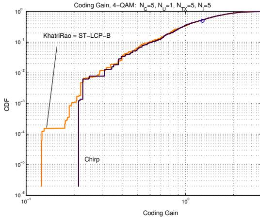
Fig. 8. CDF of coding gain: Comparison of Khatri-Rao and LSD codes
