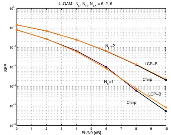
Fig. 6. SER performance: Comparison of ST-LCP and LSD codes
