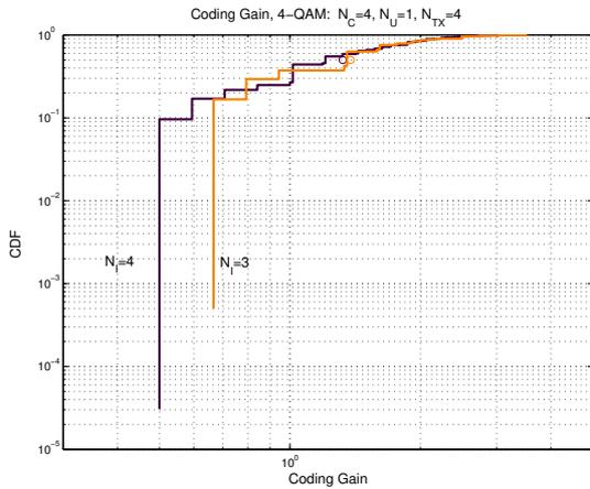
Fig. 4. CDF of coding gain: Comparison of different code rates  $r_C = \frac{N_L}{N_C}$  for LSD codes
