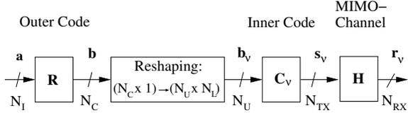
Fig. 1. Symbol discrete model of the encoding scheme
