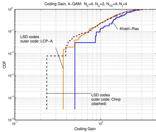
Fig. 7. CDF of coding gain: Comparison of Khatri-Rao and LSD codes
