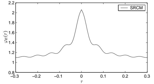
Fig. 5. Autocorrelation of the CIR energy using the SRCM.
