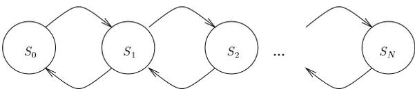
Fig. 1. State diagram of the semi-Markov process for the first model.
