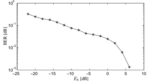
Fig. 4. Bit error rate for discrete CIR energy states ( $SNR=20$  [dB]).
