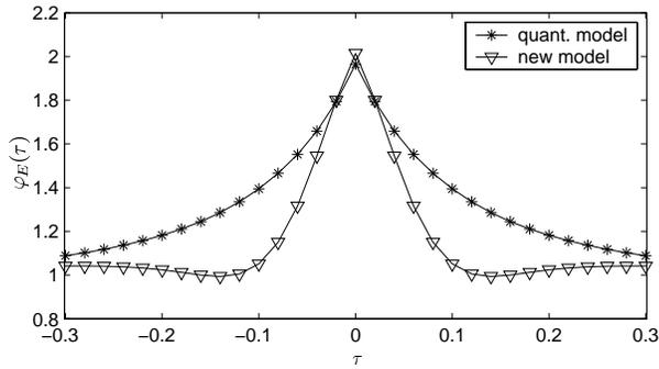
Fig. 6. Autocorrelation of the CIR energy for finite state models.
