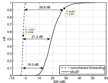
Fig. 8. cdf of the SIR at RACooN node 8 for noncoherent forwarding and MUZF.
