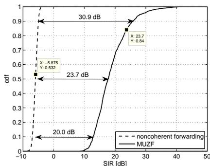
Fig. 7. cdf of the SIR at RACooN node 6 for noncoherent forwarding and MUZF.
