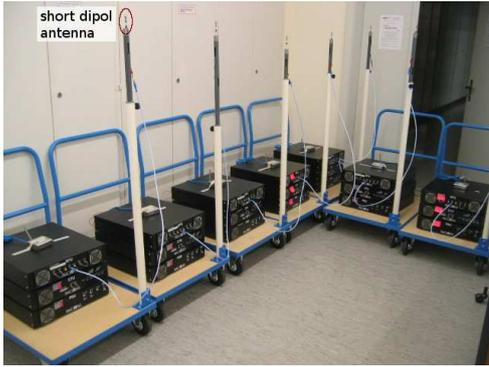
Fig. 2. 7 RACooN nodes placed on carts for mobility. The antennas are mounted at a height of about 1.5 m.
