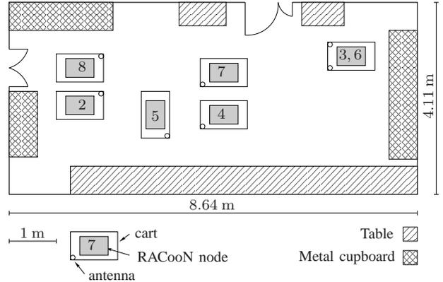
Fig. 3. Measurement setup and topology. The numbers 3–8 indicate the numbering of the RACooN nodes. RACooNs 3 and 6 are stacked on top of each other on the same cart.
