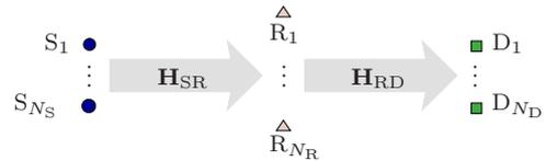
Fig. 1. Two-hop system configuration with half-duplex relays
