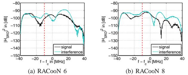
Fig. 5. Equivalent two-hop channels for noncoherent forwarding.
