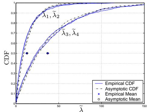
Fig. 3: Eigenvalue CDFs of the relay-assisted MIMO Rayleigh channel for  $K = 4$  relays and  $N = 20$  antennas, due to symmetrical reasons (Fig. 2) we have  $\mathbb{E}\{\lambda_1\} = \mathbb{E}\{\lambda_2\}$  and  $\mathbb{E}\{\lambda_3\} = \mathbb{E}\{\lambda_4\}$
