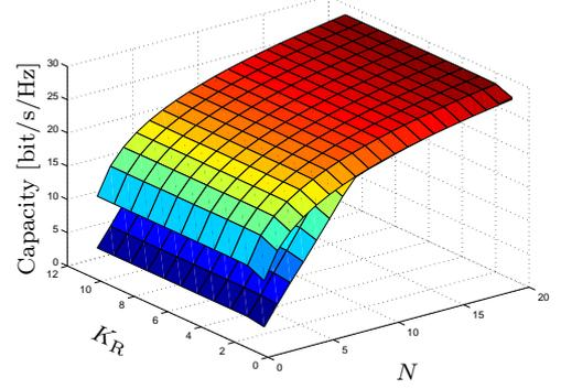
Fig. 5: Capacity of the relay-assisted MIMO Rice channel vs. Rice factor  $K_R$  and number of antennas  $N$  for  $K = 8$  relays
