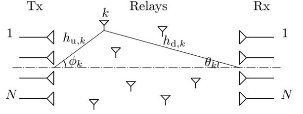
Fig. 1: Relay-assisted MIMO communication system
