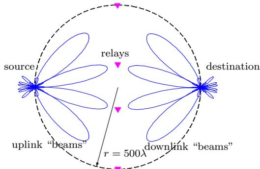
Fig. 2: Source and destination with multiple antennas, relays are single antenna nodes, at 17 GHz we have  $r = 500\lambda \approx 8.8\text{m}$
