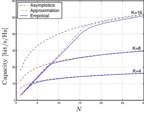
Fig. 4: Capacity of the relay-assisted MIMO Rayleigh channel vs. number of antennas  $N$  for  $K = 4, 8, 16$  relays
