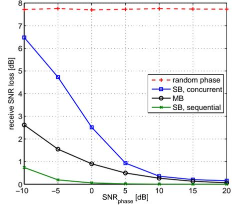
Fig. 5. Receive SNR loss due to inaccurate phase estimation
