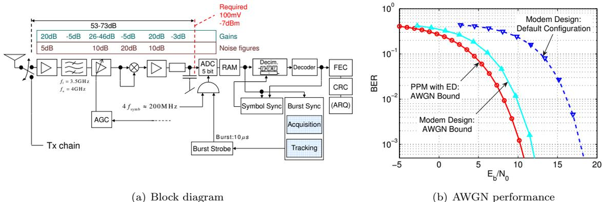
Figure 1: Modem design and performance of the UWB-ED receiver
