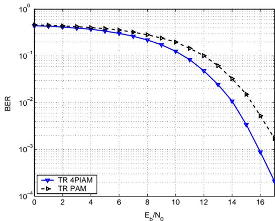
Fig. 7. Bit error ratios for NLOS channels from 0-4 meters
