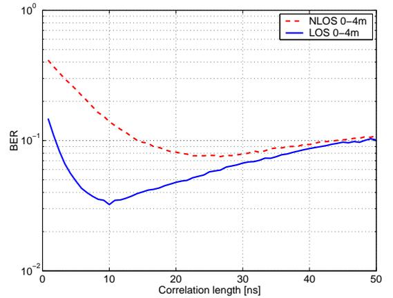
Fig. 5. Bit error ratios for TR 4PIAM with different correlation lengths ( $E_b/N_0 = 12$ dB)
