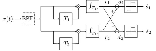
Fig. 2. Simple receiver structure for TR 4PIAM
