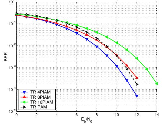
Fig. 4. Comparison of bit error ratios for AWGN channel
