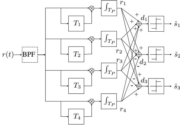
Fig. 3. Receiver structure for TR 8PIAM
