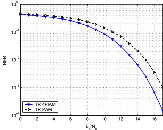
Fig. 6. Bit error ratios for LOS channels from 0-4 meters
