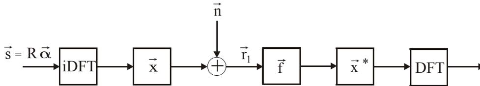
Fig. 5. Model: coded OFDM
