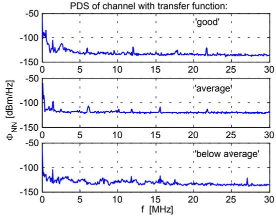
Fig. 4. Measured power density spectra (PDS) of the PLC channels in Fig. 3
