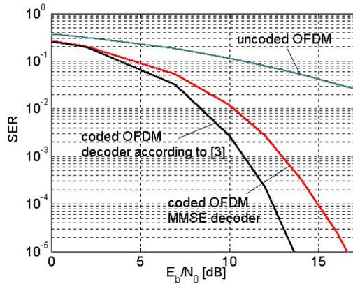
Fig. 8. Performance for PLC channel with transfer function ‘good’
