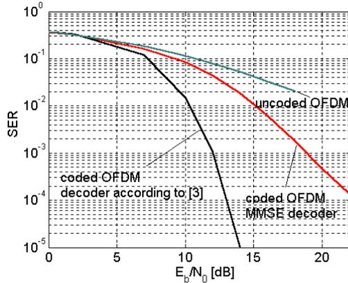
Fig. 9. Performance for PLC channel with transfer function ‘below average’
