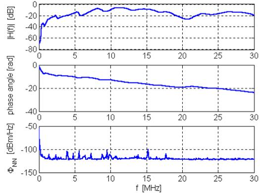
Fig. 10. Measured PLC channel (amplitude spectrum and phase angle of the transfer function, PDS)
