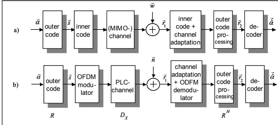
Fig. 2. Linear space-time block code (a), coded OFDM (b)
