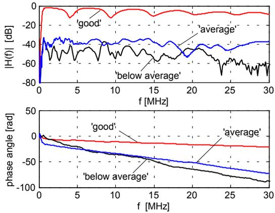
Fig. 3. Three measured PLC transfer functions (amplitude spectrum and phase angle)
