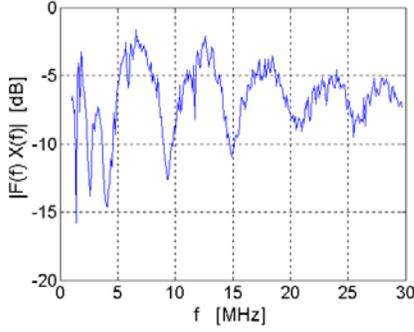
Fig. 6. Entire transfer function of PLC channel and whitening filter ('good' channel)
