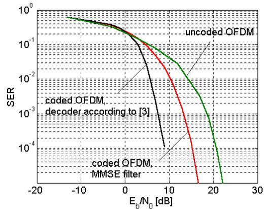
Fig. 11. Performance for the PLC channel in Fig. 9; block length 32; used frequency range 10–19.6 MHz
