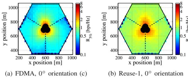
Fig. 4. 3 BSs macro diversity UB: 5% outage rate, FDMA and reuse-1,  $0^\circ$  orientation.
