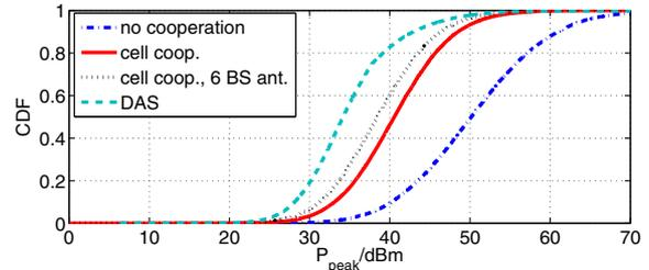
Fig. 7. CDF of max. Tx power of 3 cooperating BSs, target rate 1 bps/Hz, reuse-1,  $30^\circ$  orientation (BSs with  $N_B = 6$  as reference for the DAS case).
