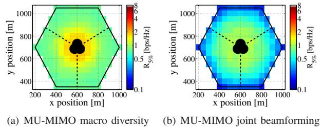
Fig. 6. MU-MIMO: 5% outage rate, frequency reuse-1, 12 omnidirectional antennas.
