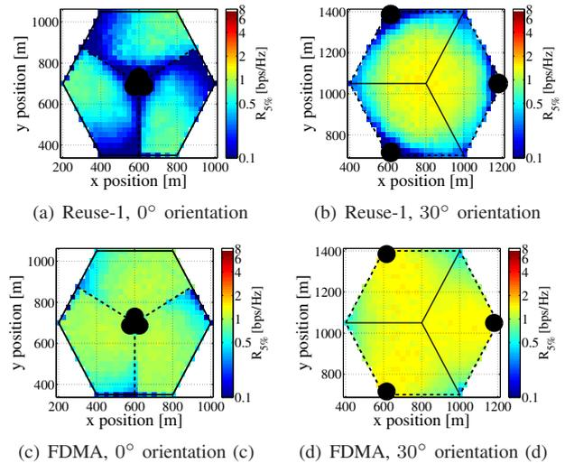
Fig. 3. Cooperation of 3 BSs: 5% outage rate, reuse-1 or FDMA.
