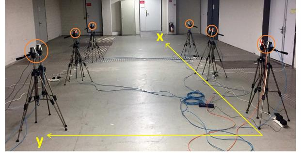
Fig. 2: Photo of the gate with six anchors (orange markers) as used in the later scenarios. For four-anchor operation, unused devices were switched off.
