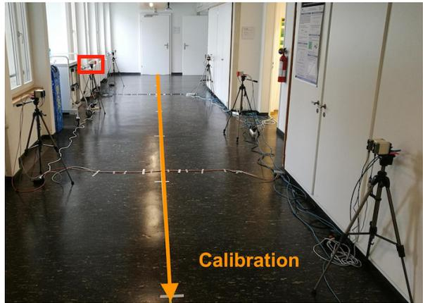
Fig. 8: Anchor constellation for the corridor setup.
