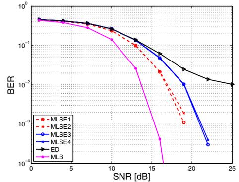
Fig. 5. BER for weak ISI (Max. Excess Delay = 14 ns)
