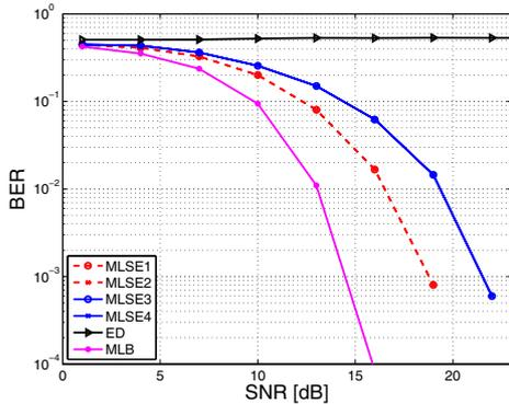
Fig. 8. MLSE for synchronization (Max. Excess Delay = 8 ns)
