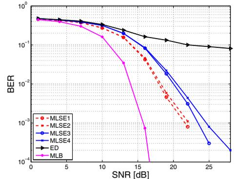
Fig. 6. BER for strong ISI (Max. Excess Delay = 17 ns)
