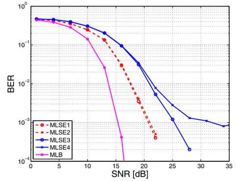
Fig. 9. MLSE for synchronization (Max. Excess Delay = 14 ns)
