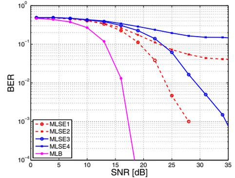
Fig. 10. MLSE for synchronization (Max. Excess Delay = 25 ns)
