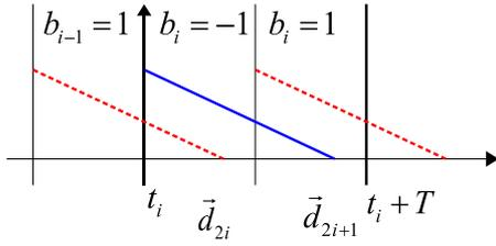
Fig. 1. ISI due to large channel excess delay
