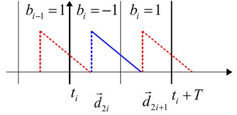
Fig. 3. ISI due to synchronization error.
