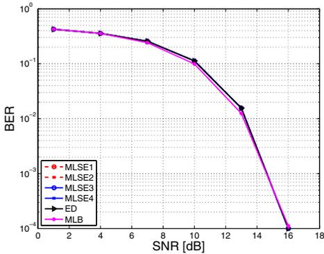
Fig. 4. BER in case of no ISI (Max. Excess Delay = 8 ns)
