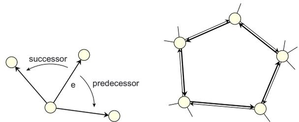
Fig. 2. On the left side, the definition of the successor and predecessor of the edge  $e$  is displayed. On the right side, the constructed face and its edges are marked with thick lines.
