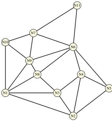
Fig. 4. Fiber topology according to the COST 239 case study for a Pan-European Network.
