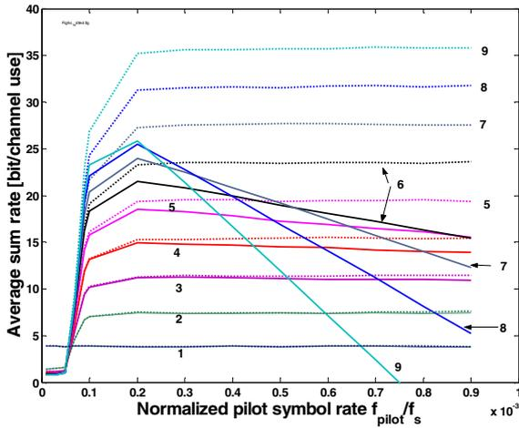
Fig. 10: Impact of a time-variant channel matrix on the average sum rate of the *minimum relay*  $N_a$  configuration. The x-axis gives the normalized pilot symbol rate, parameter of the curves is the number of source/destination pairs. The dashed lines take into account one channel use to measure and disseminate both channel matrices, the solid lines take into account  $2N_a$  channel uses to measure and  $2N_a N_r$  channel uses to disseminate both channel matrices.
