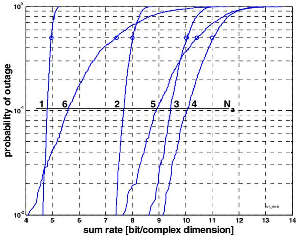
Fig. 4: Cumulative density function (CDF) of the sum rate of a  $(N_a \times 31 \times N_a)$  system with total power constraint. Parameter is the number of source/destination pairs.
