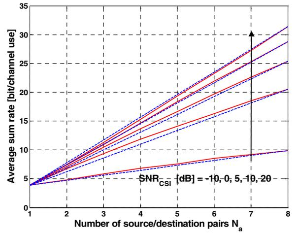
Fig. 8: Impact of noisy channel state information (CSI). We show the average sum rate of the *minimum relay*  $N_a$ -configuration versus the number of source/destination pairs. Parameter of the curves is the excess SNR of the CSI.
