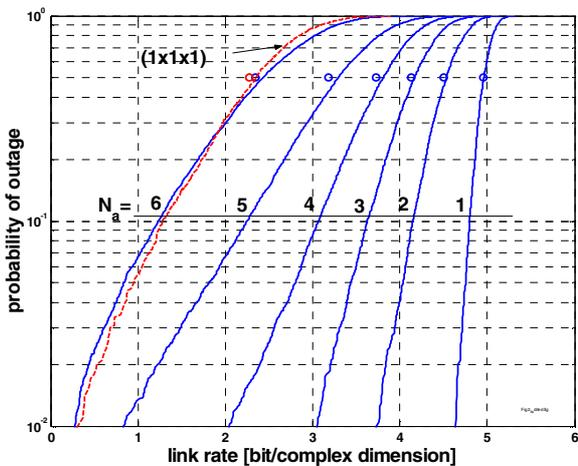
Fig. 5: CDF of the link rate of a  $(N_a \times 31 \times N_a)$  system with link power constraint.
