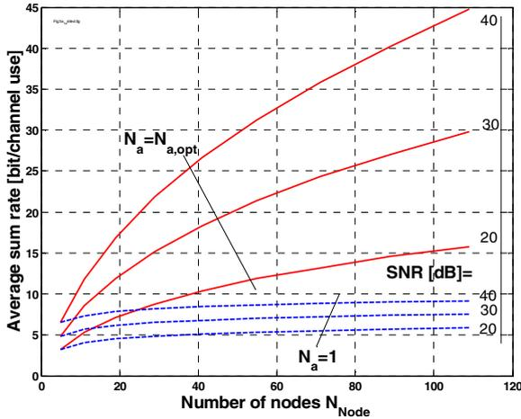
Fig. 7: Maximum average sum rate versus the total number  $N_{node}$  of nodes in the network. Parameter is the SNR. For reference the dashed curves give the performance of a  $(1 \times N_{node} - 2 \times 1)$  configuration.
