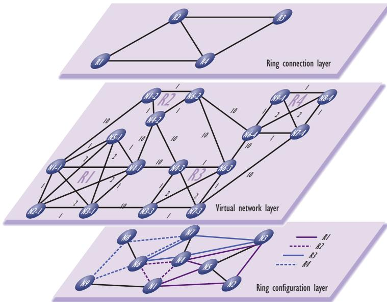
which is referred to as the ring configuration layer, contains the real network nodes and the real fibre topology. The actual configuration is a set of rings. Each ring consists of a set of nodes and edges of the network. A 'face' is the smallest possible ring in a network. By using the face concept, it is possible to construct rings in a systematic way with low complexity. The enlargement of a ring involves adding further faces, while shrinking is achieved by deleting faces.<sup>8</sup>
